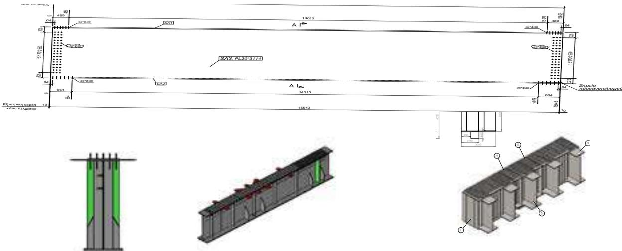
The bridge is supported by four ball bearings in reinforced concrete plinths, each of which is grounded in an array of 6 holes 1,20m in diameter and 15,00m deep. Its connection to the land area is made by joints with the possibility of moving up to 40cm in the longitudinal direction of the bridge.
