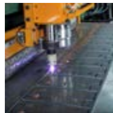
The Oxy/Fuel torch delivers CNC accuracy on 75 mm thick plate.
