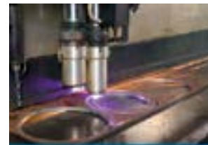
A powerful Plasma unit delivers high speed, accurate contoured cuts.
