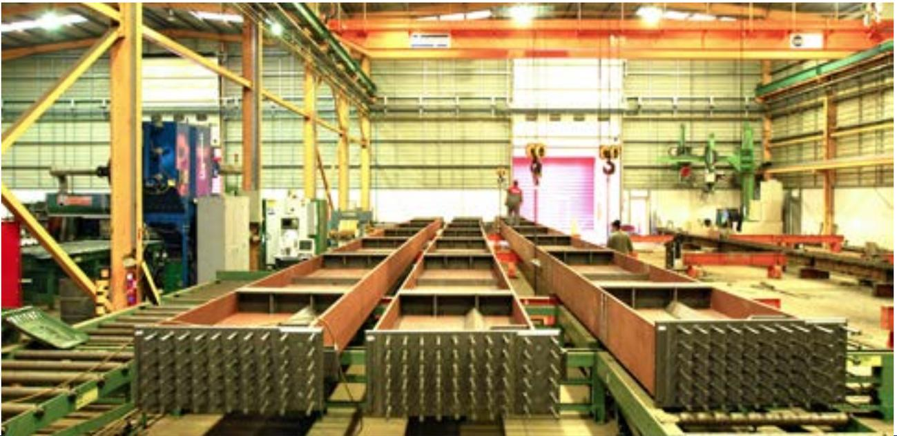
Basic element without a union concerned the length of the beams ~ 30m, benefiting from increased strength, road transport, reduction of erection time and reduced maintenance requirements.
